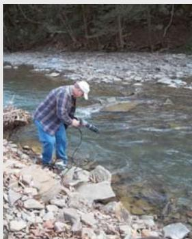
Dr. Barnard holds the monitor (a YSI-6600 V2-4 sonde) that is submerged in Silver Creek. It transmits data (eg, conductivity, turbidity), via a solar-powered cell phone, to Wilkes Univ. computers.
